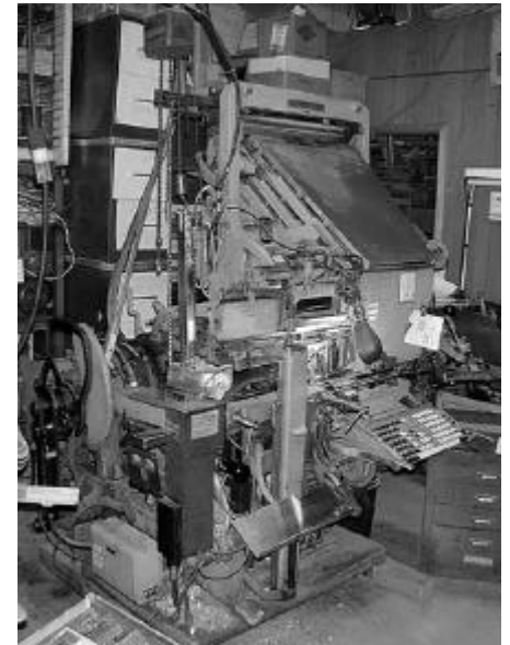
A massive and complex Intertype machine similar to the ones Don Black serviced in his early days. The operator would sit beneath the keyboard located near the bottom right. The machine generated lead type in a line to be placed on the printing press.
