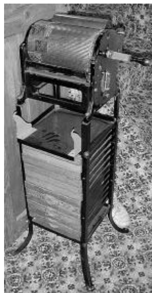
There were many printing devices designed over the years. This was one of them. The print drum had grooves which fit specially designed elements stored in the drawers beneath, and the paper ran beneath the drum.
