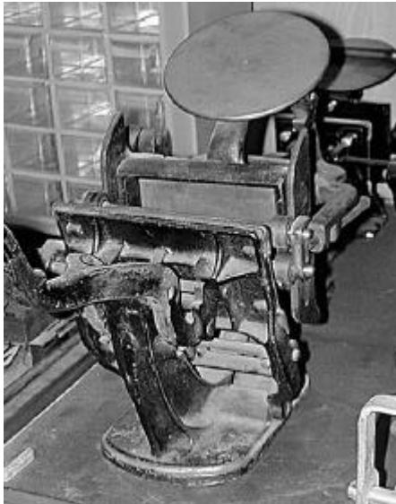
A smaller table-top platen press (sometimes called a clamshell press, which describes the way it opens and closes on the type). These were sometimes used as hobby presses, or in companies that printed their own stationery or cards.
