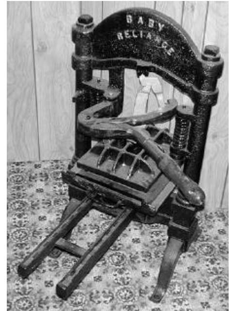
A miniature version of the large iron standing press, the Baby Reliance might just manage a business card.
